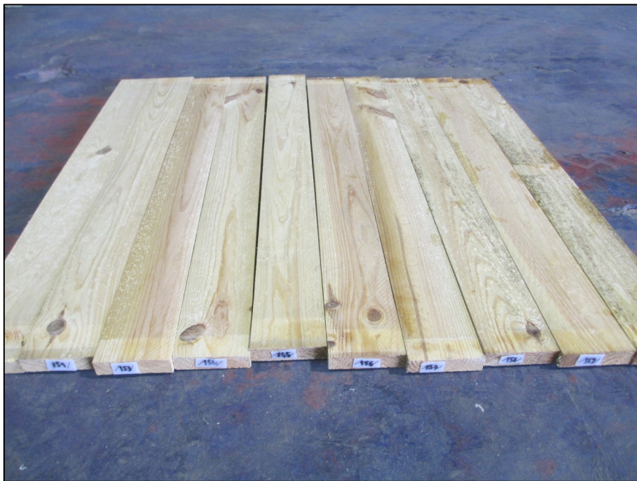
Figura 3 Samples of wood treated with the solution F 2530/2 (2%), open stacked – Grading: 1,62
