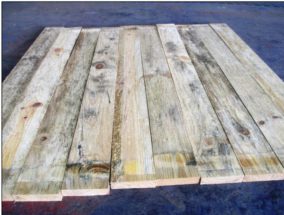
Figure 7 Samples of the untreated wood – open stacked - Grading: 3,95
