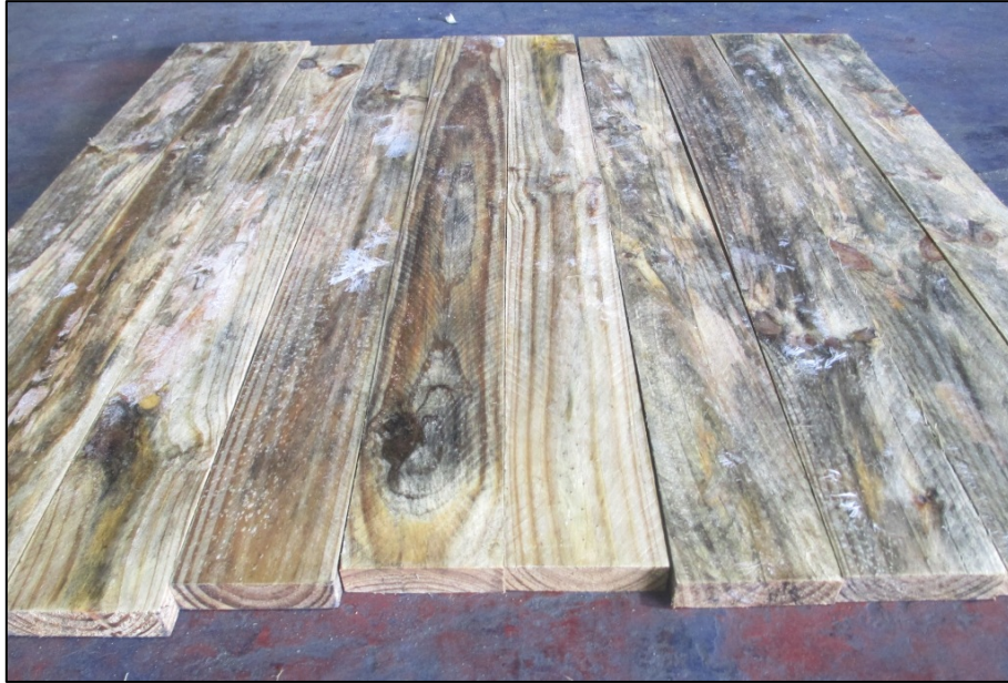
Figure 6 Samples of the untreated wood – close stacked – Grading: 4
