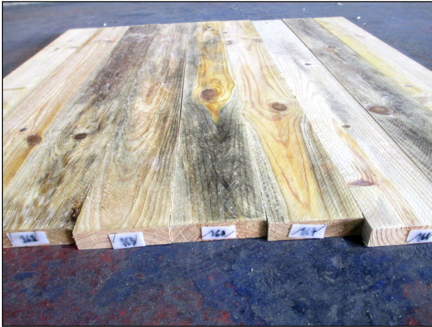
Figure 11 Samples of wood treated with the solution Celbrite FS1 (10%), close stacked – Grading: 3,03
