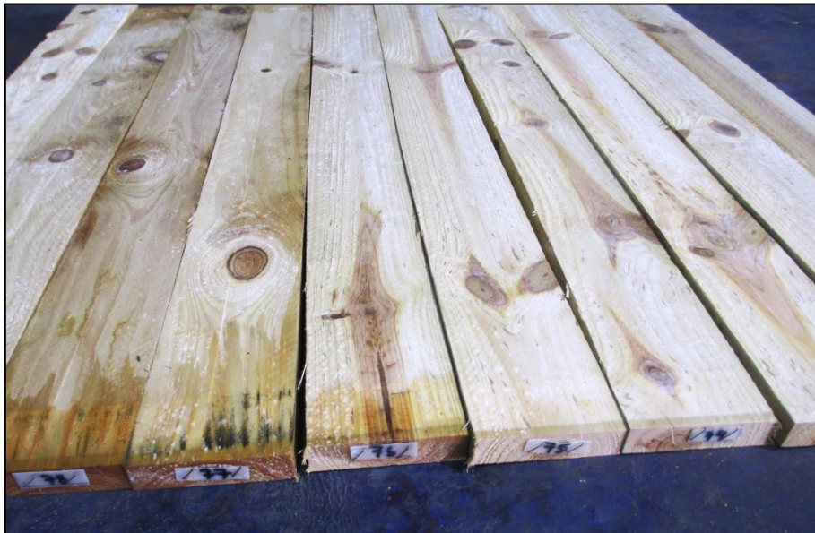
Figure 10 Samples of wood treated with the solution Corpol Madera Verde (4%), open stacked – Grading: 1,06
