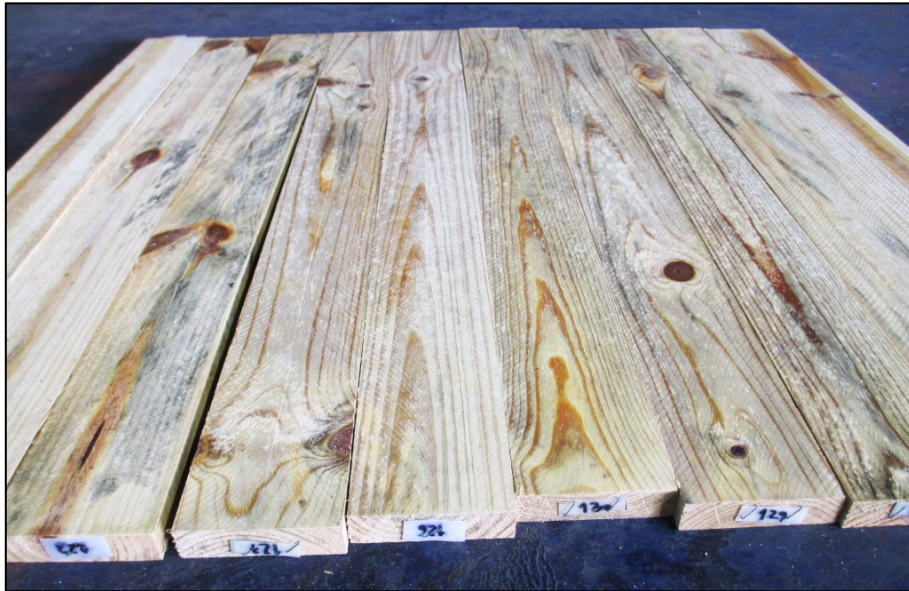
Figura 4 Samples of wood treated with the solution F 2530/2 (1%), close stacked – Grading: 2,91
