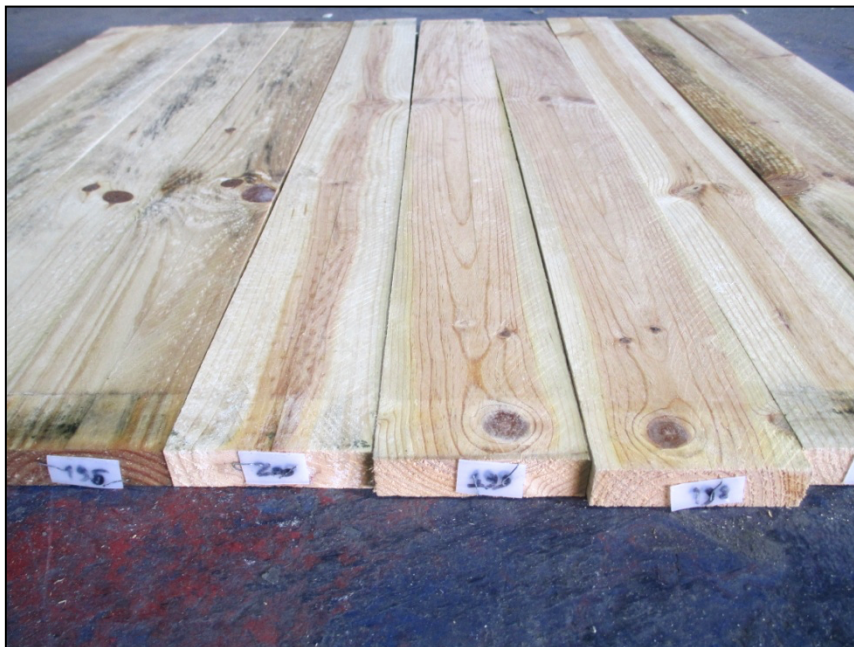
Figure 14 Samples of wood treated with the solution Celbrite FS1 (15%), open stacked – Grading: 2,08
