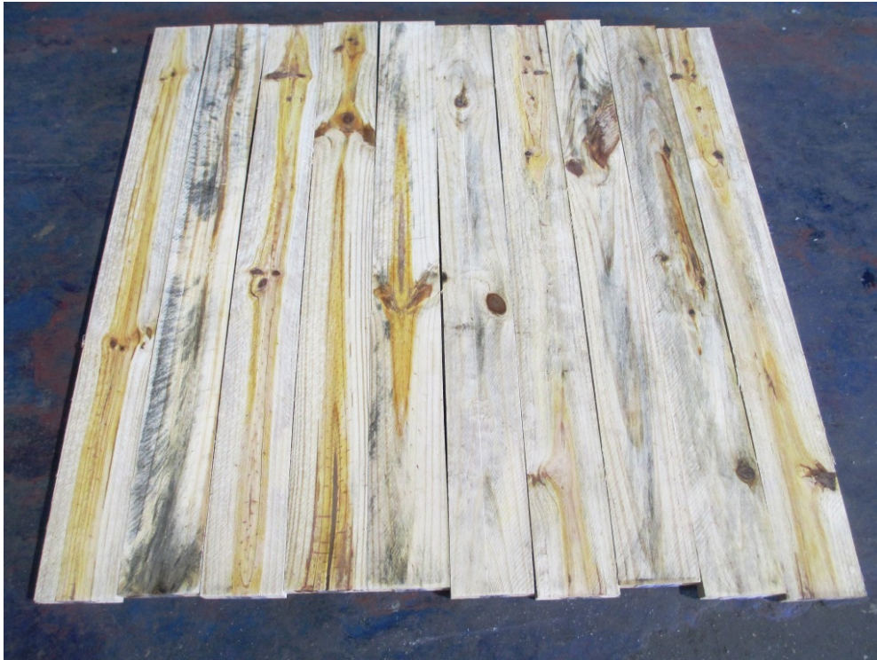
Figure 8 Samples of wood treated with the solution Antiblu Select 3787, close stacked – Grading: 3,18
