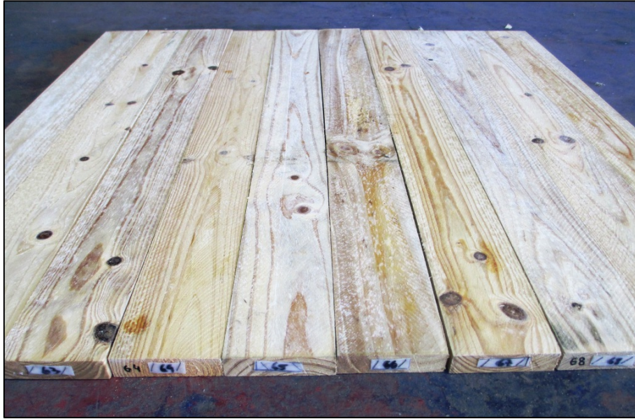
Figure 9 Samples of wood treated with the solution Corpol Madera Verde (4%), close stacked – Grading: 1,24
