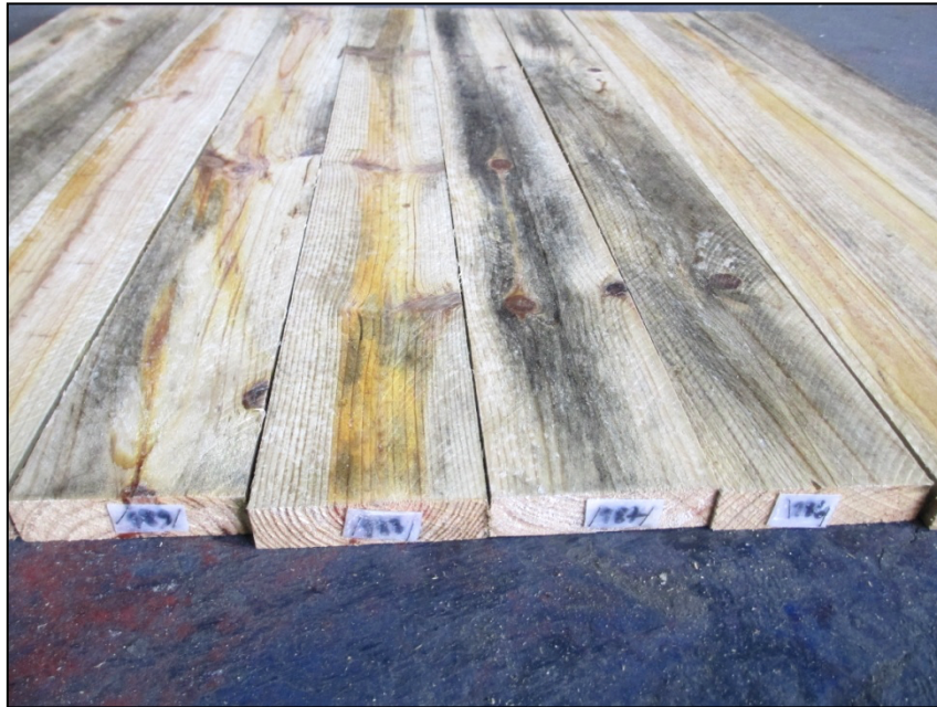
Figure 13 Samples of wood treated with the solution Celbrite FS1 (15%), close stacked – Grading: 3,68
