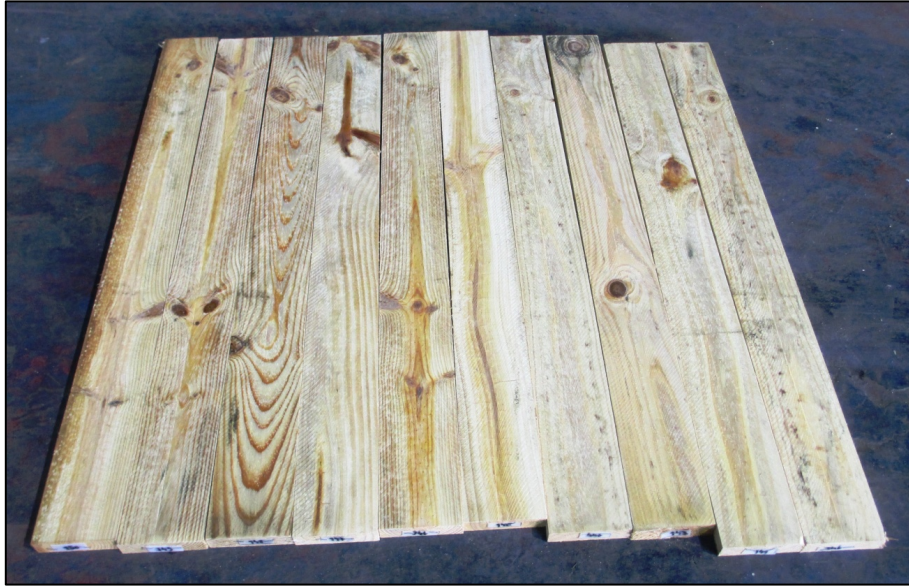
Figura 2 Samples of wood treated with the solution F 2530/2 (2%), closed stacked – Grading: 2,50
