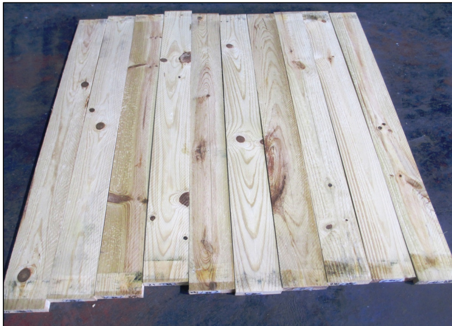
Figura 1 Samples of wood treated with the solution Antiblu Select 3787, open stacked – Grading: 1,33
