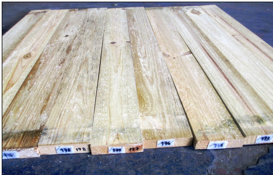
Figure 12 Samples of wood treated with the solution Celbrite FS1 (10%) open stacked – Grading: 1,95
