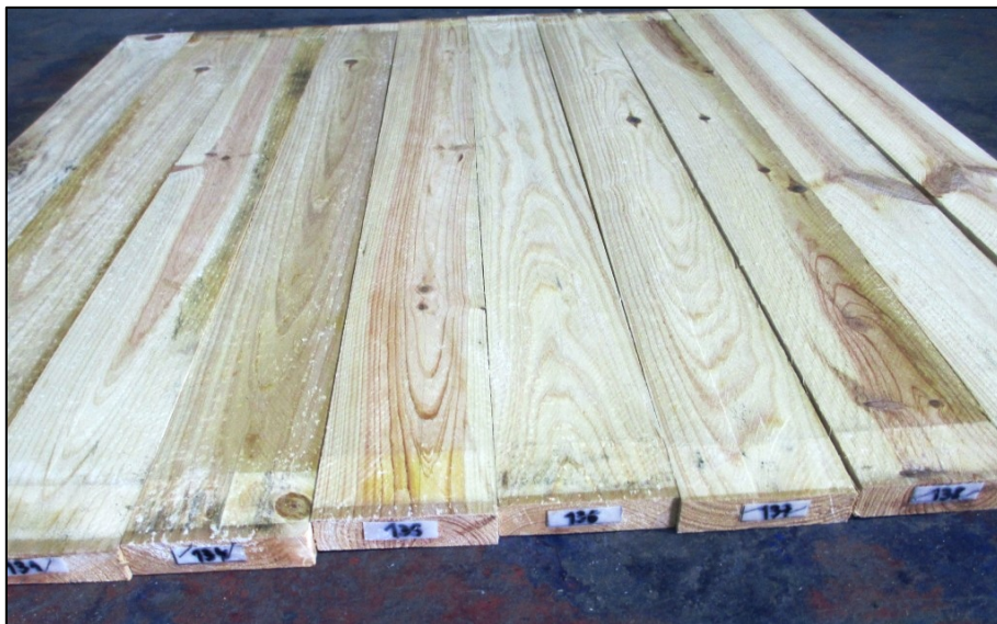
Figura 5 Samples of wood treated with the solution F 2530/2 (1%), open stacked – Grading: 1,30
